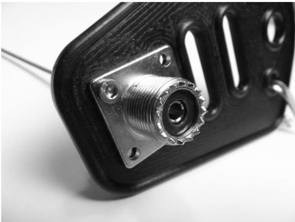
Thread the steel wire with SO-239 from the front securing the SO-239 temporarily with one screw.
