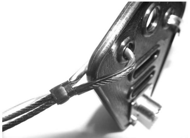
Add a ferrule to the wire (moving it down to the rear of the SO-239) then thread through centre feed plate and around the thimble from the rear to the front. Align the wire with thimble guides then thread back through the ferrule. Position the ferrule as tight and close to thimble as possible leaving a good size loop between the thimble and the SO-239. TIP: hold the ferrule in your crimper and pull both wires as tight as possible for a neater finish.
